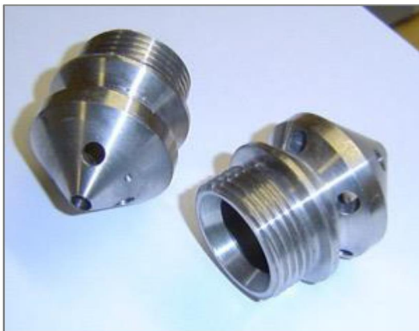
Victor nozzles for fitting to 1" dia. lance. [2]
