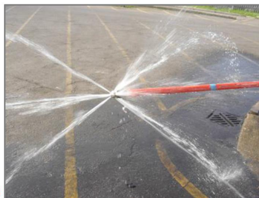
Victor nozzle spray pattern (red lance – blue depth marker). [2]
